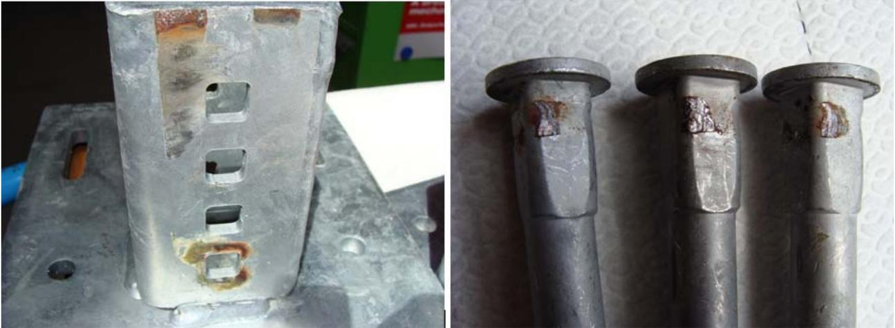
**Fig. 10: Wear in the sliding parts due to abrasion (Test #2).**
