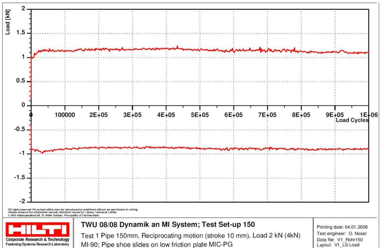
Fig. 7: Load graph of Test #1 over 1 million cycles.
