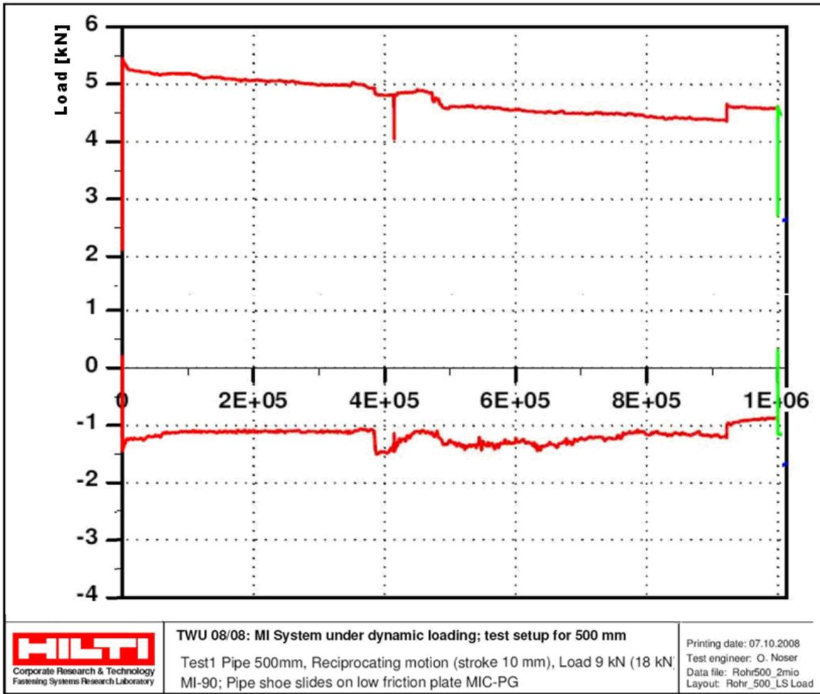
Fig. 8: Load graph of Test #2 over 1 million cycles.
