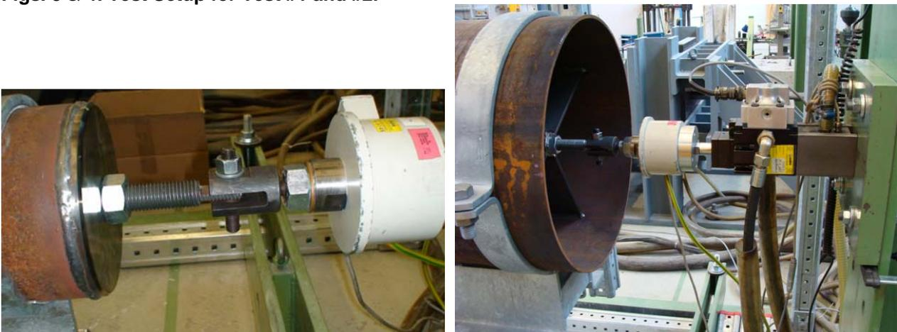
Figs. 5 & 6: Coupling between pipes and dynamometer for Test #1 and #2.
