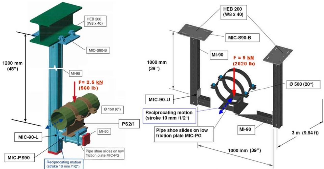
Figs. 1 and 2: Test #1 and Test #2 Setup.
