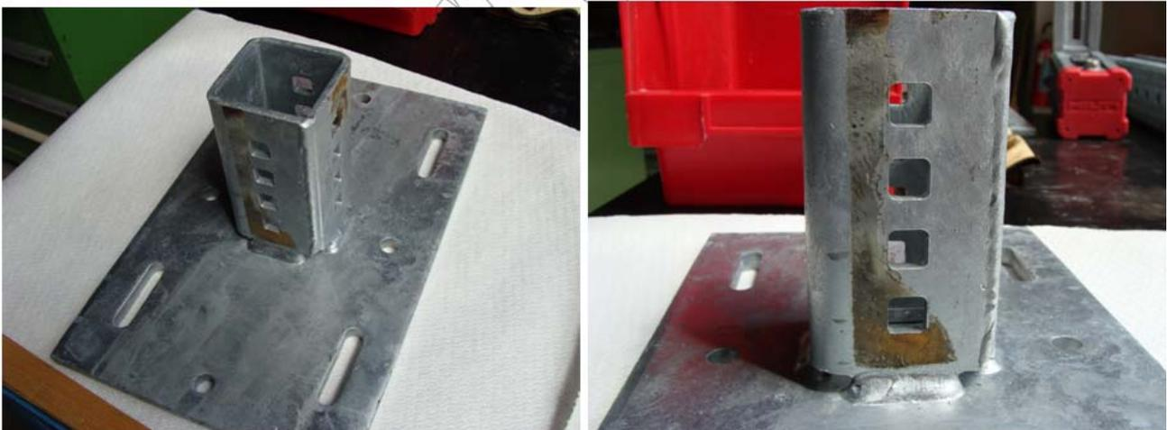
Fig. 9: Wear in the sliding parts due to abrasion (Test #1).
