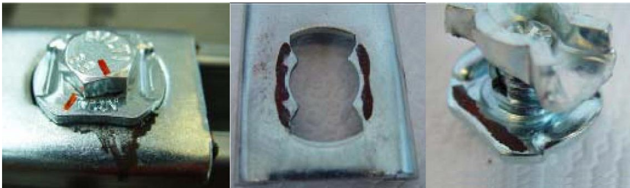
Fig. 4: Condition of push button and connection after 50'000 cycles.
