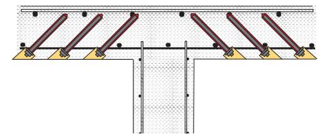
Fig. 2 Post-installed punching shear reinforcement applied only from bottom side of the slab
