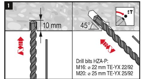
A special drilling stand is available on request for guided drilling under 45° angle with higher precision and comfort.
