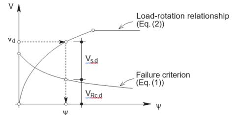
Fig. 11 Load on slab and concrete shear resistance
