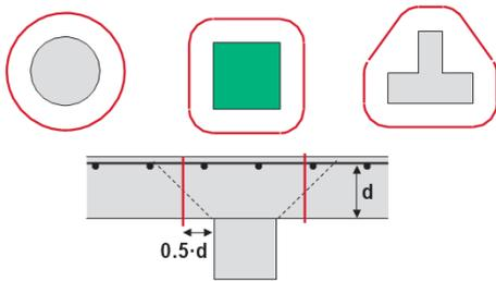
Fig. 12 Shear perimeter  $u_o$  for typical column shapes
