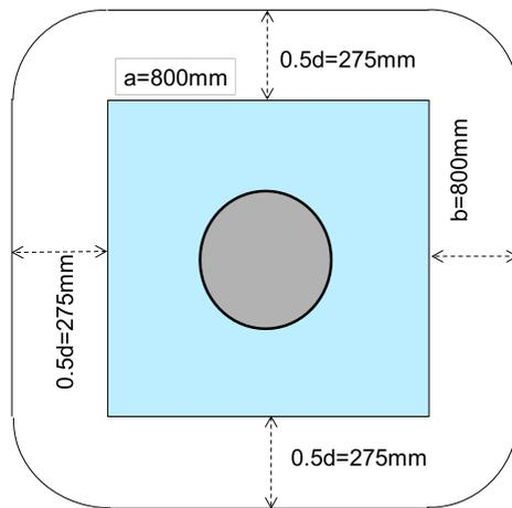
The punching shear resistance  $V_{Rd,c} = 2366 \text{ kN}$  is lower than the acting shear load  $V_d = 4109 \text{ kN}$ . Therefore, the slab must be strengthened.
