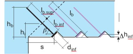
Fig. 13 geometry of reinforcement
