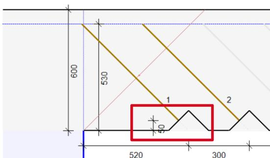
Fig. 22 Visualization of  $\Delta h_{inf}$  in Design report
