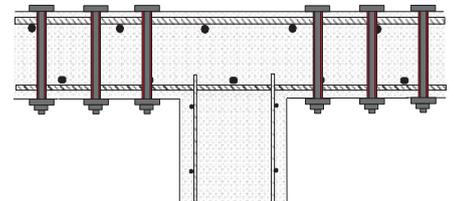
Fig. 1 Penetrating post-installed punching shear reinforcement
