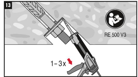
Fig. 33 Injection of mortar into washer
