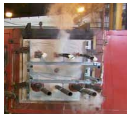
Fire test after seismic impacts
