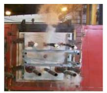
Fire test after seismic impacts
