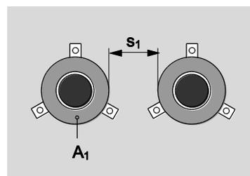
**Sound decoupling:** Sound decoupling strips (C<sub>1</sub>) based on combustible insulation (elastomeric foam, e.g. PE) minimum E (acc. to EN 13501-1), used in combination with gypsum plaster or mortar as gap filler. Sound decoupling installed around the pipe within the wall. For maximum thickness see tables below.
