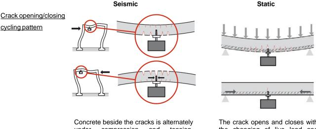
Concrete beside the cracks is alternately under compression and tension, resulting in the worst conditions for the anchor zone. The crack opens and closes with the changing of live load and rebar restrain, which is less severe compared to seismic conditions
