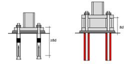
Due to the complexity of defining loads for capacity design and the extreme difficulty of achieving ductile anchor failure in the application, the elastic design approach is often used for base plate application design.
