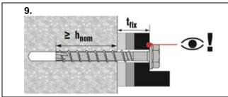
The anchor can be adjusted max. two times.
