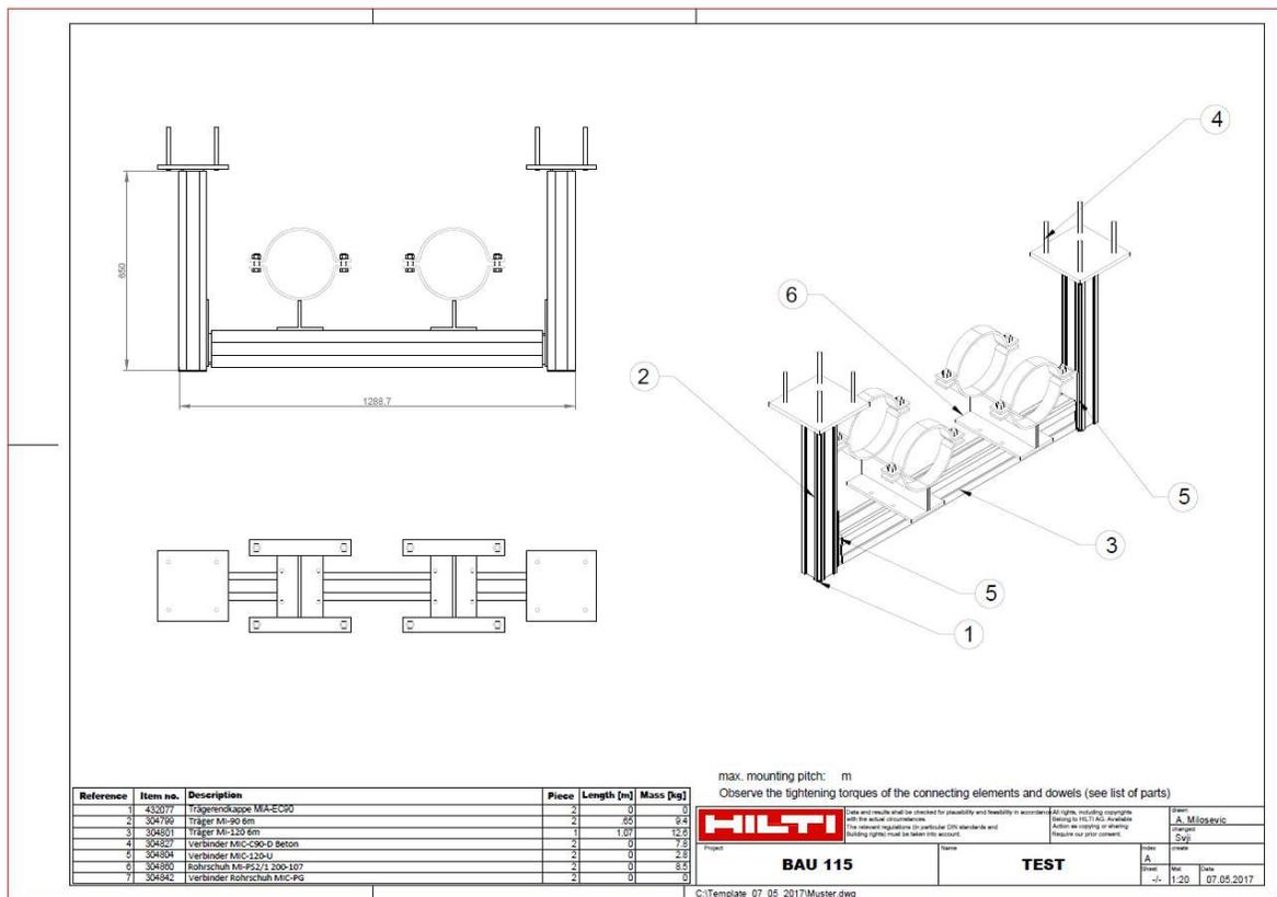
Fig.4: Sample AutoCAD 2D / 3D shop-drawing
