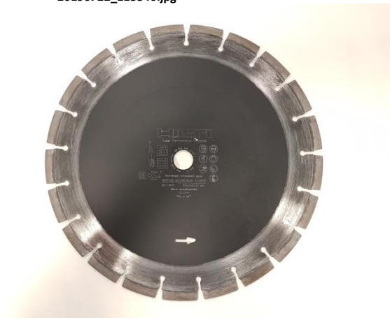
Figure 1 Hilti DCH 300-X diamond cutter (Top left), Hilti VC 40-UM vacuum unit (top right), and Hilti SP-S 305/22 Univ 305 mm diameter diamond blade (bottom)
